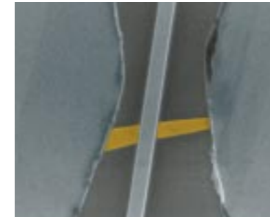
Graphen-Transistor mit 1 \mu\text{m} Top Gate Graphene transistor with 1 \mu\text{m} top gate
